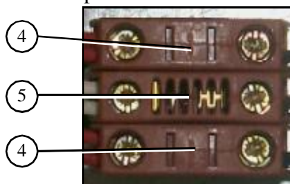
Detailed view of a two position switch.
